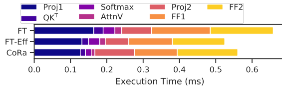
Figure 24. Breakdown of execution times of the encoder layer for the CoLA dataset at batch size 32 on the GPU.
