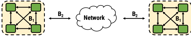
Figure 7: An example 2-level hardware topology. Solid green boxes represent GPUs. Each server (dashed yellow boxes) has 4 GPUs connected internally by links of bandwidth B_1 ; each server is connected by links of bandwidth B_2 . In real systems, B_1 > B_2 . Figure best seen in color.
