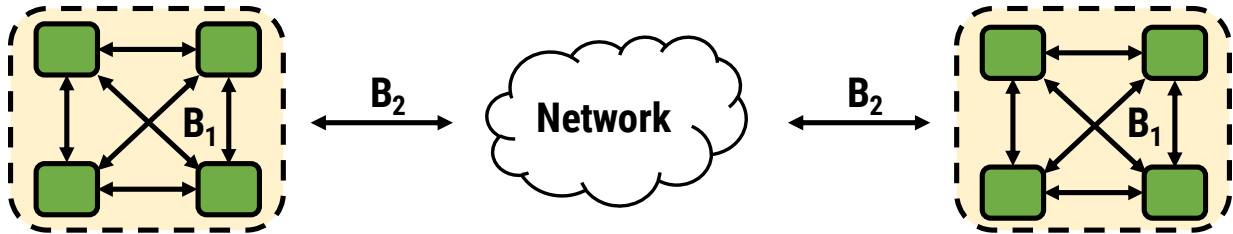
Figure 5.7: An example 2-level hardware topology. Green boxes represent GPUs. Each server (yellow boxes) has 4 GPUs connected internally by links of bandwidth B_1 ; each server is connected by links of bandwidth B_2 . In real systems, B_1 > B_2 .
