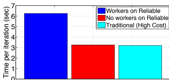
Figure 4.10: AgileML stage 1 with 4–32 reliable machines out of 64 total compared to traditional (all 64 reliable; cyan), for MF.
