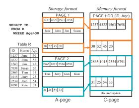
Figure 1: Decoupled storage device and in-memory layouts.
