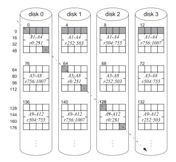
Figure 5: Mapping of a database table with 12 attributes onto *Atropos* logical volume with 4 disks. The numbers to the left of disk 0 are the *LBNs* mapped to the gray disk locations connected by the arrow and not the first block of each row. The arrow illustrates efficient semi-sequential access fetching single A-page with 63 records. A single sequential I/O for 16 *LBNs* can efficiently fetch one attribute from 1008 records striped across four disks.
