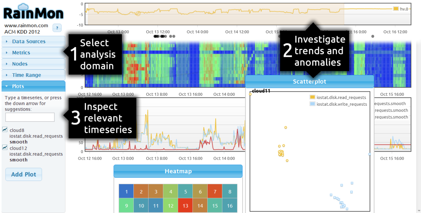
Figure 7: RainMon interface. Overlaid in black boxes is the workflow of the tool. At bottom are the scatterplot of W_{:,2} vs W_{:,1} and a machine “energy” heatmap. In the central pane are linked, zoomable, customizable timeseries plots. An interactive demonstration of the interface is available at http://demo.rainmon.com .
