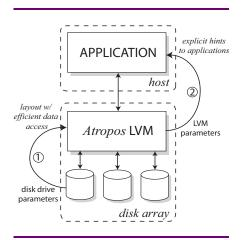
Atropos logical volume manager architecture. Atropos exploits disk characteristics (arrow 1), automatically extracted from disk drives, to construct a new data organization. It exposes high-level parameters that allow applications to directly take advantage of this data organization for efficient access to one- or two-dimensional data structures (arrow 2).
