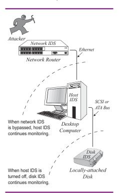
The role of a disk-based intrusion detection system (IDS). A disk-based IDS watches over all data and executable files that are persistently written to local storage, monitoring for suspicious activity that might indicate an intrusion on the host computer. IDS functionality in low-cost desktop disk drives.
