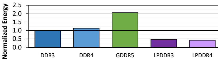
Fig. 26. Mean DRAM energy consumption for common OS routines, normalized to DDR3.
